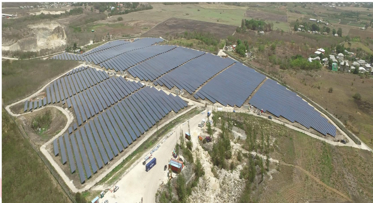
Picture 1: Ariel view of the 10 MW PV solar farm of BL&P (source: Greaves and Gill, no year, slide 10)
